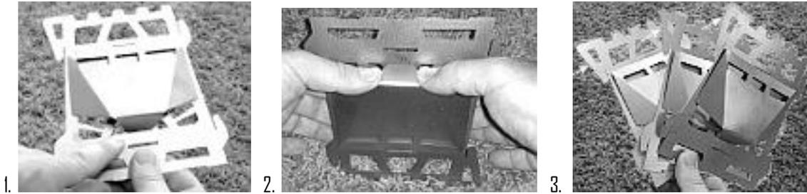
1. Install the afterburners into all side panels. The top tab goes in the slot at the top of the side panel. The bottom goes into the damper plate support hole.
